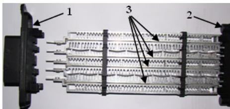
Fig. 8. PTC heater components
