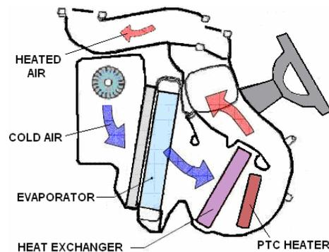
Fig. 6. Air flow inside the HVAC
