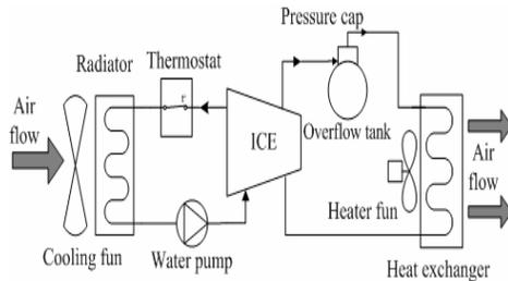
Fig. 1. Liquid cooled system
