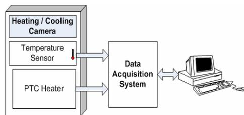
Fig. 10. Test bench scheme implementation
