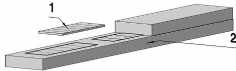
Fig. 9. PTC Heating resistive elements
