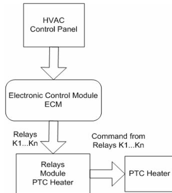
Fig. 7. PTC heater control
