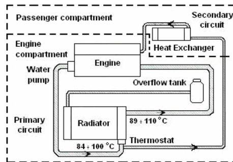
Fig. 2. Diagram of a cooling system
