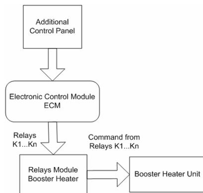
Fig. 4. *Booster heater control diagram*
