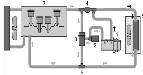
Fig. 5. *Integration of a booster heater in the ICE cooling system* [16]
