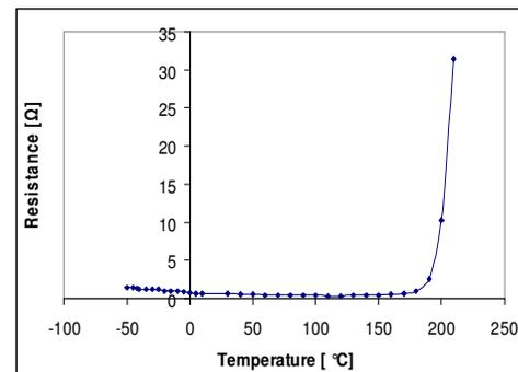
Fig. 12. Resistance - Temperature characteristic curve of 900 W PTC heaters
