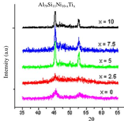
Fig. 8. X ray diffractograms recorded for  $Al_{79}Si_{11}Ni_{10-x}Ti_x$  ( $x = 0...10$ ) compositions
