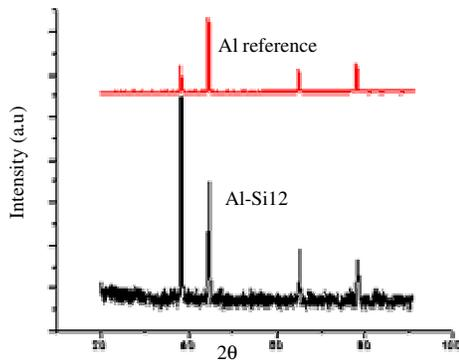
Fig. 5. X ray diffractograms for the Al-Si12 composition
