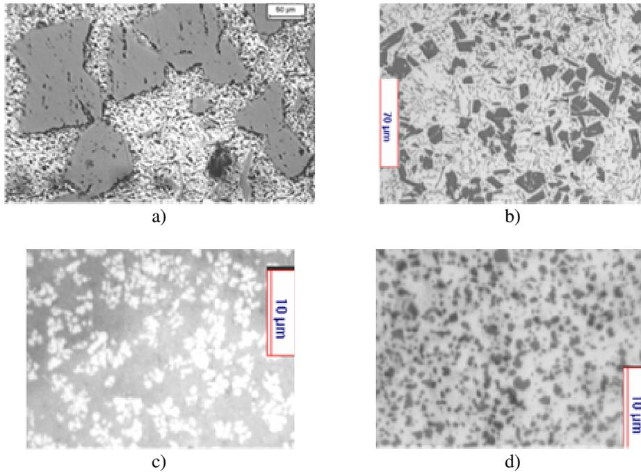
Fig. 6. Quantitative and qualitative modifications determined by the increase in the cooling rate, in the case of a hypereutectic silumin  $Al_{80}Si_{20}$ :
