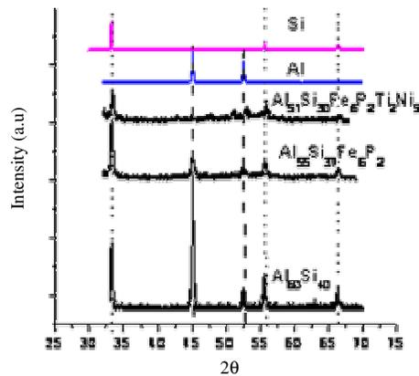
Fig. 9. X ray diffractograms recorded for compositions based on the Al-Si40 system
