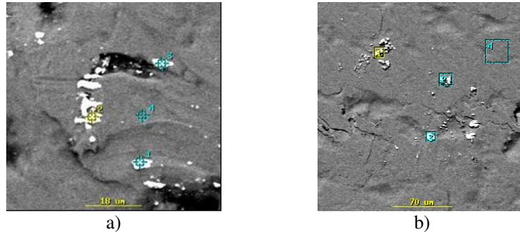
Fig. 7. Defect points on the smooth surface of Al-Si20 ribbons, with increased concentrations of alloying elements in points 1, 2 and 3: a) iron and b) zinc
