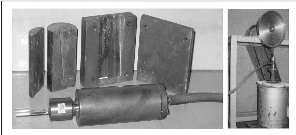
Fig. 2. Devices for the high cooling rate processing of aluminium based alloys:
