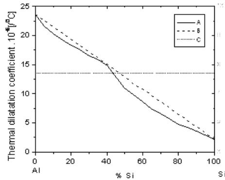
Fig. 1. Variation of the thermal dilatation coefficient in the Al-Si system compared to the motor cylinder:
