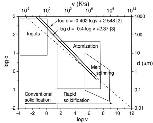
Fig. 4. Interdependence: Cooling rate vs. Dendrite parameters [6-8]
