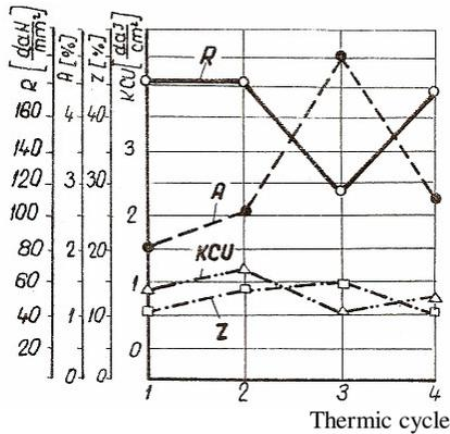
Fig. 2. Variation of mechanical properties depending on thermic cycle
