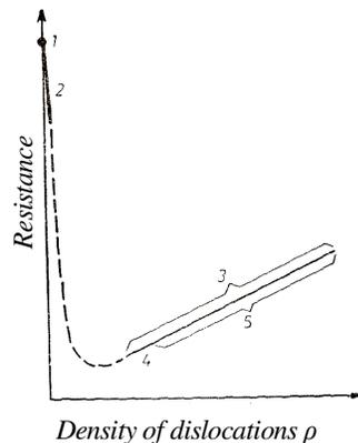
Fig. 1. Variation resistance depending on density of dislocations: 1 - theoretical resistance; 2 - resistance of filiform crystals; 3 - the real resistance of materials and alloys; 4 - resistance of non cold hammered materials; 5 - resistance of cold hammered materials and alloys
