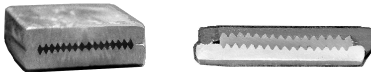
Fig. 14. Cold welded samples with intermediate cogged layer
