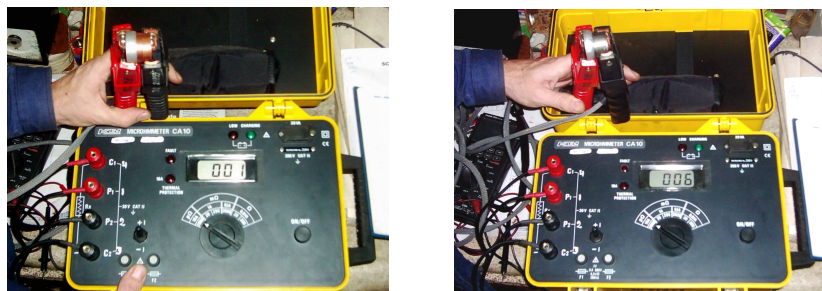
Fig. 12. Contact electric resistance measurements
