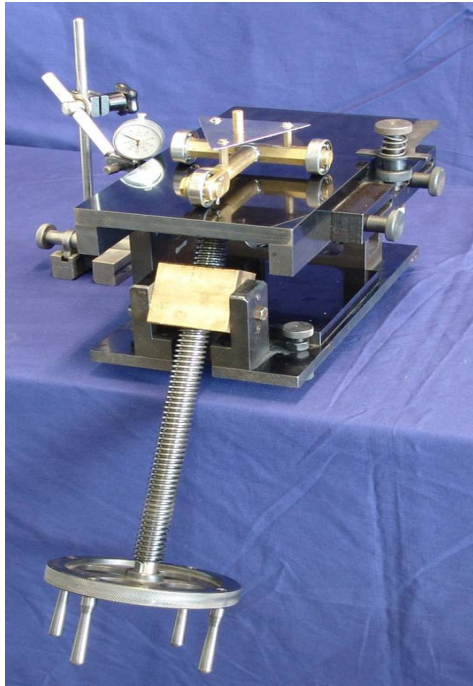
Fig. 1. Mechanical system consisting of a device of three radial bearings and a high-precision tribometer
