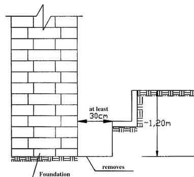
Fig. 6. *Removing the soil till foundation base, for a minimum 30 cm wide distance*
