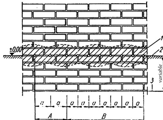
Fig. 1. Treatment with synthetic resins:
