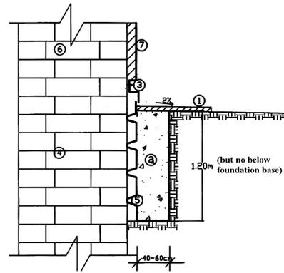
Fig. 7. *Detail for ventilating foundation at “Adormirea Maicii Domnului” church*
