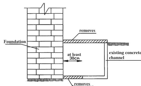
Fig. 5. *Removing the bottom channel for a minimum 30 cm wide distance*
