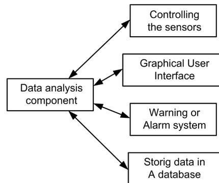
Fig. 2. *The software structure of a geodesic monitoring system*
