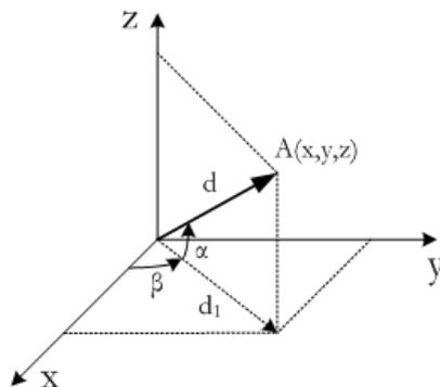
Fig. 3. Transformation of polar coordinates into cartesian coordinates
