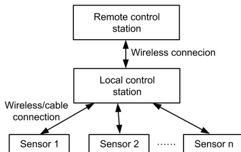
Fig. 1. *The hardware structure of a geodesic monitoring system*
