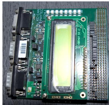
Fig. 7. *Mini robot's CPU*
