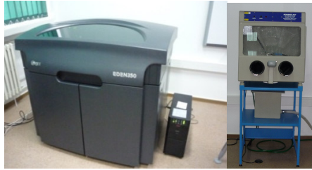
Fig. 5. EDEN 350 printer and its water jet recycle station - Transilvania University of Braşov
