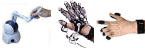
Fig. 2. Force feedback and tactile feedback devices
