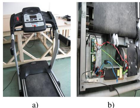
Fig. 2. *Energetics Power Run 3000 HRC* - structure (a) DC motor, control module (b)
