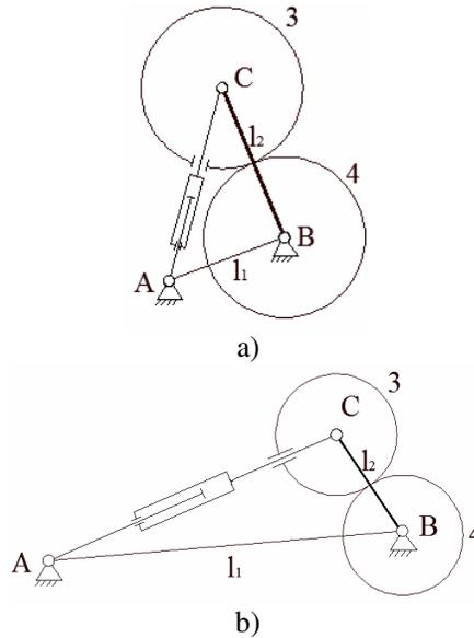
Fig. 2. Two types of the geared linkage: a)  $l_1 < l_2$ ; b)  $l_1 > l_2$
