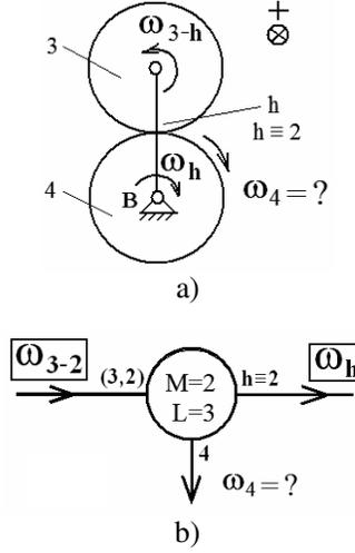
Fig. 4. a) Differential planetary gear pair and its b) black box scheme
