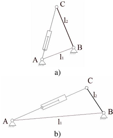
Fig. 1. Two types of the triangle linkage driven by a linear actuator: a)  $l_1 < l_2$ ; b)  $l_1 > l_2$
