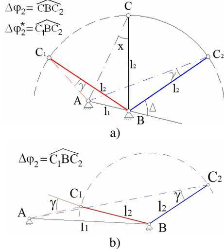
Fig. 3. a) Initial and final position of the linkage for minimum admitted  $\gamma$  and intermediary position for maximum  $\gamma$  ( $\gamma_{\max} = x$ ) when  $l_1 < l_2$ ; b) Initial and final position of the linkage when  $l_1 > l_2$
