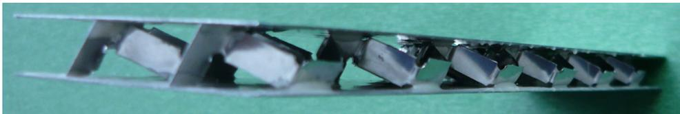
Fig. 8. *Sample of the resulted sandwich structure with the proposed cellular core made of stainless steel type 304 metal sheets*
