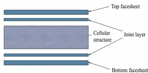
Fig. 1. *The components of a sandwich assembly*
