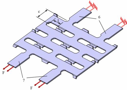
Fig. 4. *The perforated sheet material before the expansion process*
