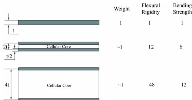
Fig. 2. Comparison between homogeneous and sandwich cross-sections [12]
