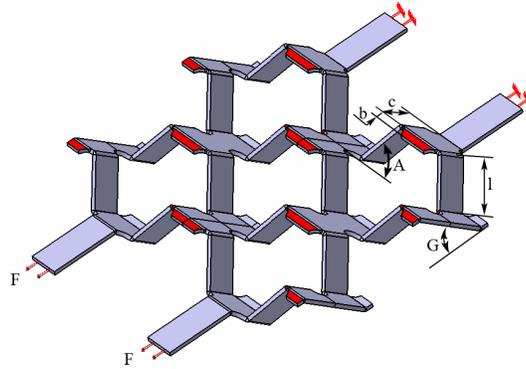
Fig. 6. *The resulted cellular core, after the expansion process*
