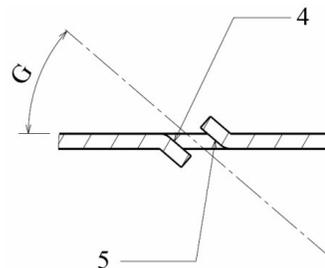
Fig. 5. *The contact surfaces of the core with the face sheets*
