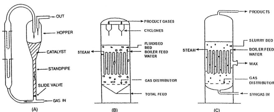
Fluidised bed FT reactors: (A) CFB reactors; (B) ebulating or FFB reactor; (C) slurry phase bubbling bed reactor
