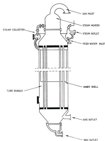
Fig. 2. *Multitubular fixed bed FT reactor* [5]
