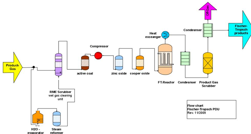
Fig. 5. The Fischer-Tropsch pilot plant flow chart [8]
