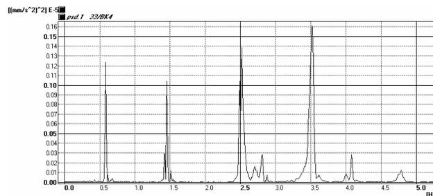
Fig. 8. *The peaks in PSD function correspond to the frequencies 0.52; 1.45; 2.50; 3.52 Hz*
