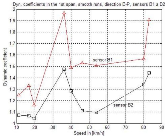
Fig. 6. Dynamic coefficients versus speed of vehicle motion
