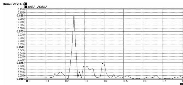
Fig. 7. *The 1st sharp peak in PSD function corresponds to the 1<sup>st</sup> natural frequency*
