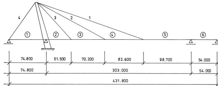
Fig. 2. Basic dimensions of the bridge
