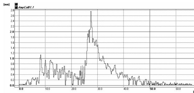
Fig. 4. Two-amplitudes of 1<sup>st</sup> span bridge vibration
