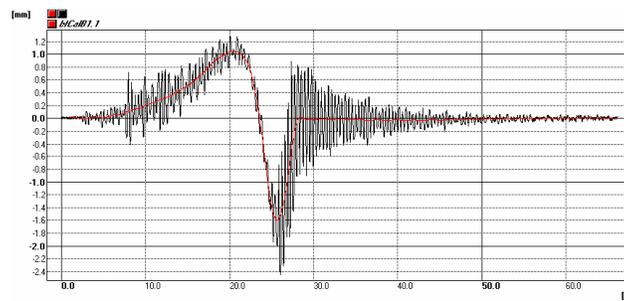
Fig. 3. Typical time record of vibration, driving direction B - P
