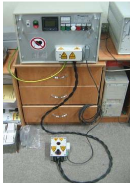
Fig. 3. The impulse magnetizer system with magnetizing coil and NdFeB sample
