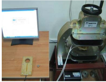
Fig. 2. Permagraph L with vertical electromagnet and NdFeB sample
