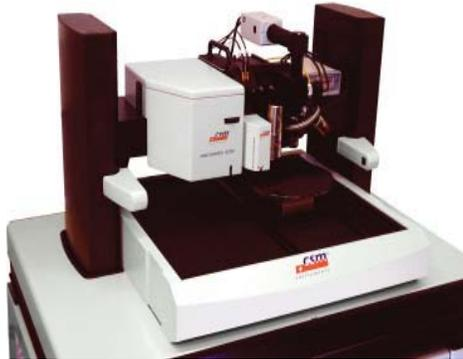
Fig. 4. Modern Nanoindentation Platform, CSM Instruments type [37]
