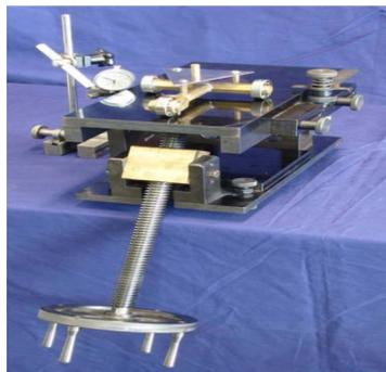
Fig. 5. Mechanical system consisting of a device of three radial bearings and a high-precision tribometer [5]
