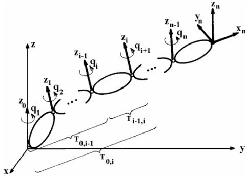
Fig. 2. Forward recursive relations on the basis of Vukobratović ( $T_{i-1,n}$  ( $i = 0, \dots, n-1$ )) homogenous transformation matrix,  $Z_{0...i}$  coordinate axis
