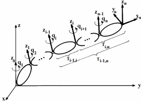
Fig. 1. Backward recursive relations on the basis of Vukobratović ( $T_{i-1,n}$  ( $i = 0, \dots, n-1$ )) homogenous transformation matrix,  $Z_{0...i}$  coordinate axis
