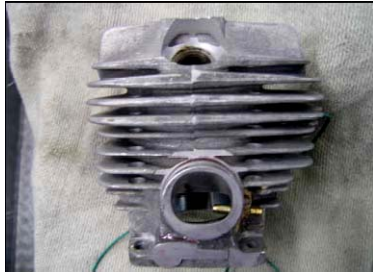
Fig. 2. Modified engine cylinder for engine lubrication [1]
