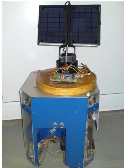
Fig. 6. *The hardware of the sun tracking system*
