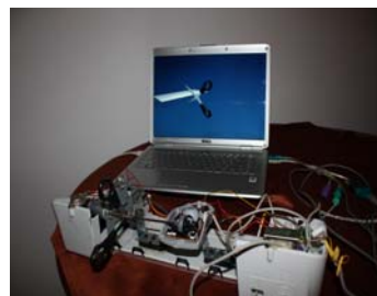
Fig. 4. Scissors device (bottom-side of the picture) and virtual scissors prototype (up-side of the picture)
