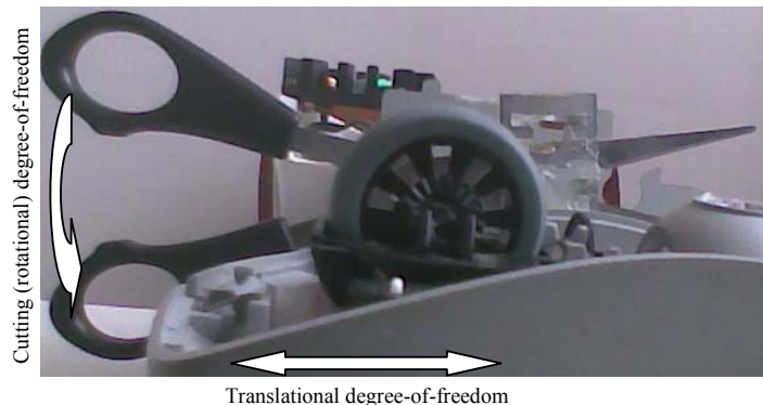
Fig. 3. Two-degree-of-freedom haptic scissors
