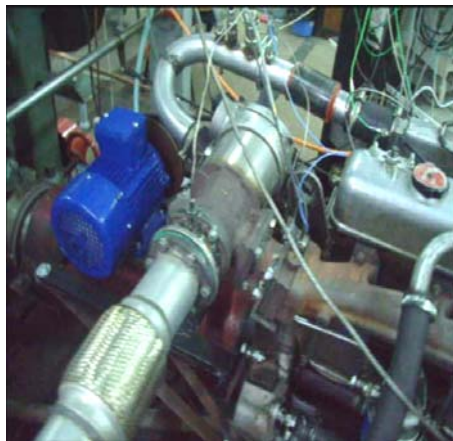
Fig. 6. Engine 392 L4 DT equipped with aggregate of type Comprex, mounted on the test bench
