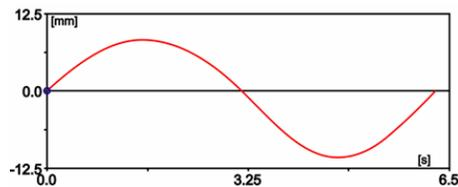
Fig. 6. Initial wheel track deviation
