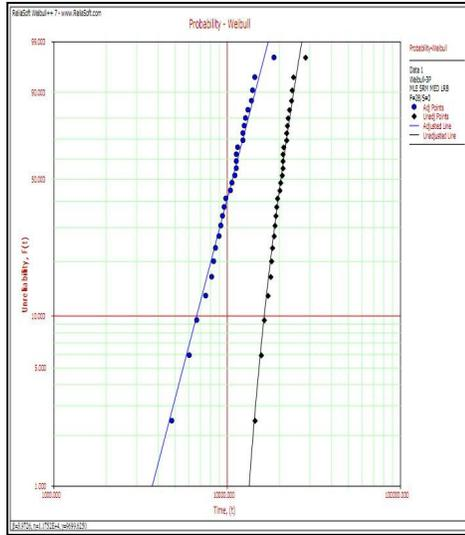
Fig. 1. Probability Plotting for 3 parameter Weibull distribution
