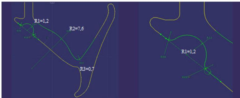
Fig. 5. Geometrical details of the original model for the inner waist belt - Model 1
