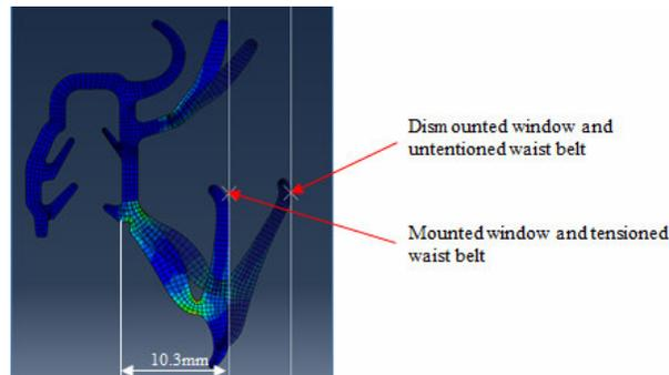
Fig. 2. *Geometrical comparison between free standing parapet and tensioned mounted parapet* [1]
