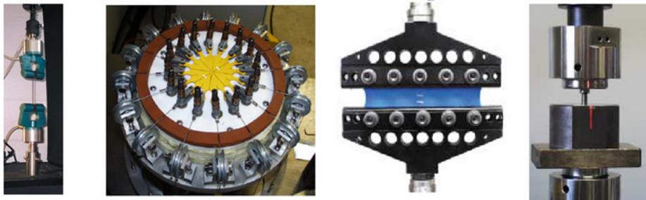
Fig. 3. Experimental methods for determining the elastic characteristics of hyperelastic materials [6]
