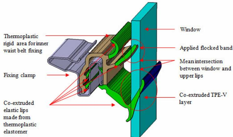
Fig. 1. *Inner door waist belt assembly - fixing method and window interaction* [2]
