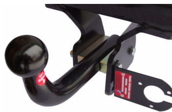
Fig. 11. Steel Structure of a towing car hook with a steel ball on the top [7]
