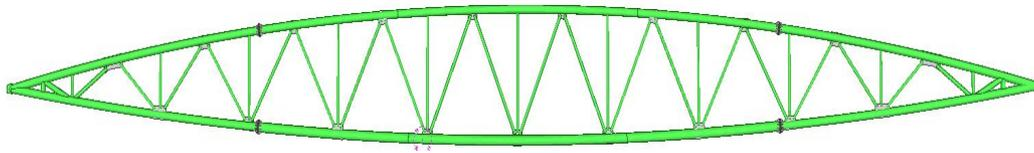
Fig. 1. *Fish-shape arched truss structure with CHS members*
