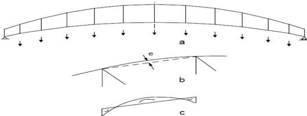
Fig. 2. *Arched trusses*
