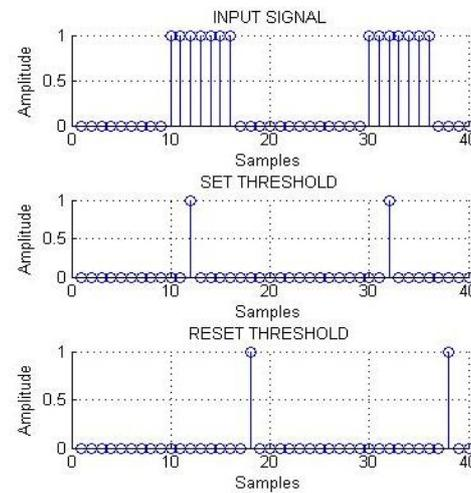
Fig. 4. *Implementation results of Bistabil function on a sampled input signal, active on the landing*
