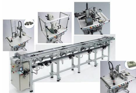
Fig. 2. *The layout of processing stations on flexible line FMS 200; ProDD Institut Braşov*
