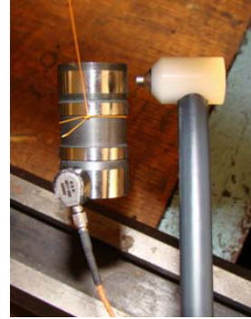
Fig. 8. Transducer placement and impact point
