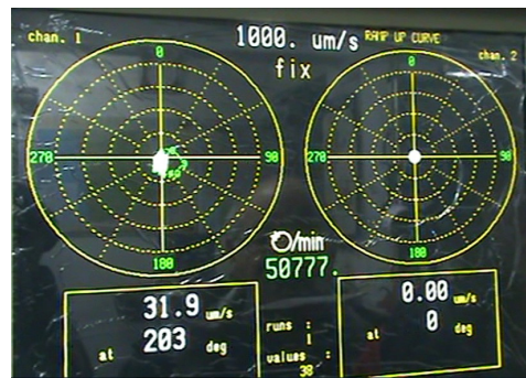
Fig. 11. Rotor precession at 50777 rpm
