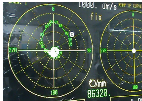
Fig. 12. Rotor precession at 86320 rpm
