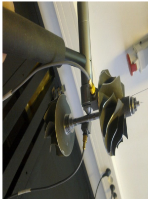
Fig. 7. Transducer and impact point for the turbocharger rotor
