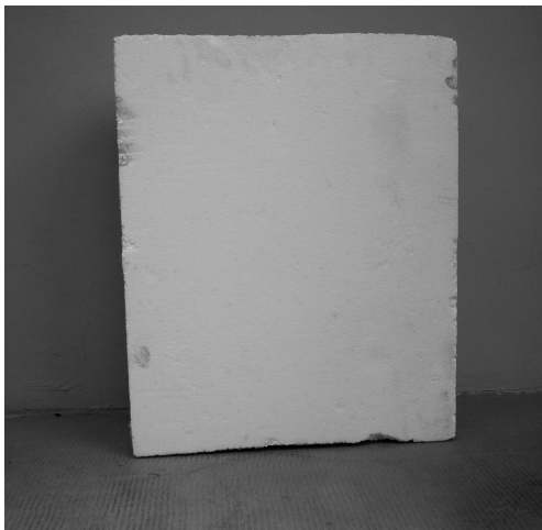
Fig. 3. Spongi-flu sound absorbing screen
