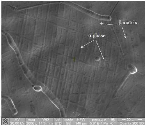
Fig. 6. SE image revealing the main phases of the as-cast titanium alloy (2000X)
