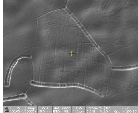
Fig. 8. SE image showing in detail a \beta grain (2000X)
