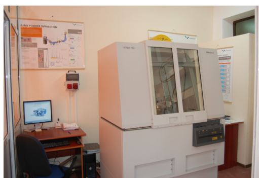
Fig. 3. X-ray diffractometer PANalytical X'Pert PRO MRD
