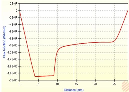
Fig. 7. *The magnetic potential simulated with Infolytica MotorSolve*
