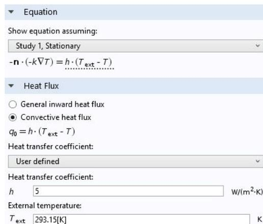
Fig. 2. Boundary conditions for the convective heat flux
