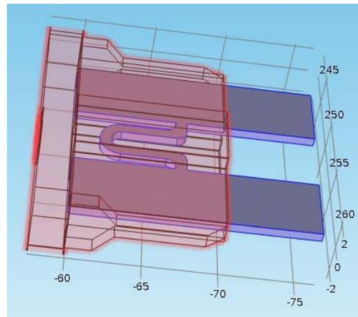
Fig. 1. *Automotive fuse 60 A, made from copper*
