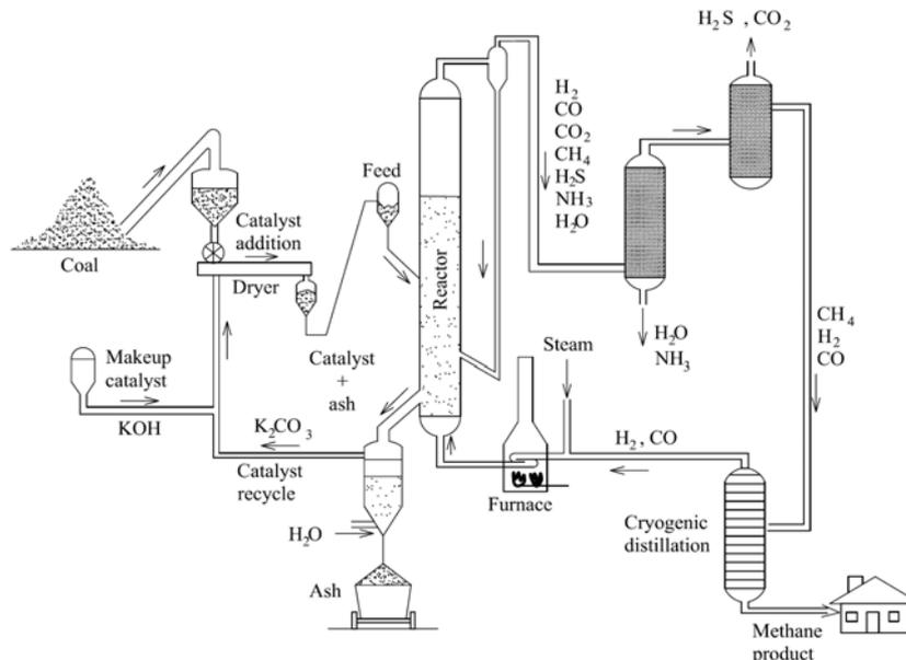
Fig. 4 The scheme of catalytic gasification process
