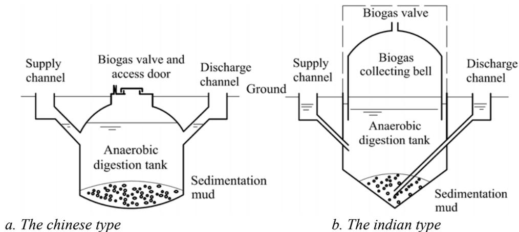
Fig. 6 Types of rural biogas reactors
