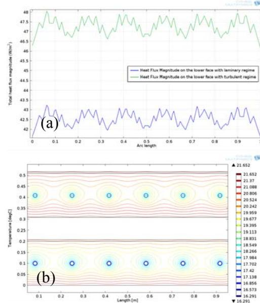
Fig.5. *The specific heat flux transferred by the lower face of the TABS (a) and tempeprature distribution (b) in case of laminar and turbulent flow*
