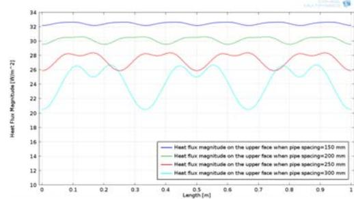
Fig.2. *Heat flux magnitude over the upper surface of the TABS for different pipe spacing*
