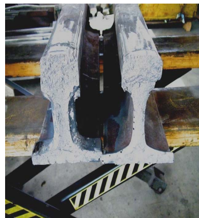
Fig. 3. The slow bending test results without modifying the sample
