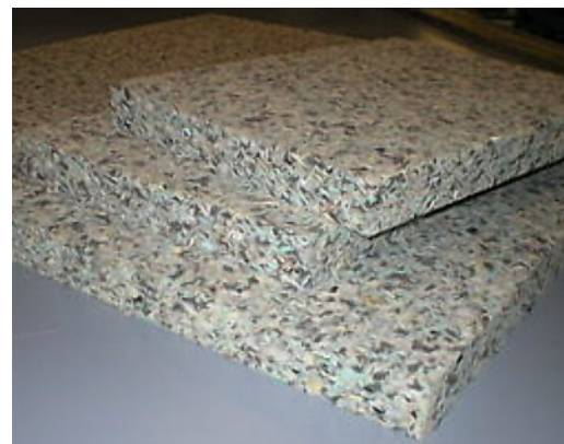
Fig. 7. Sound-absorbing panel from concrete with rubber particles
