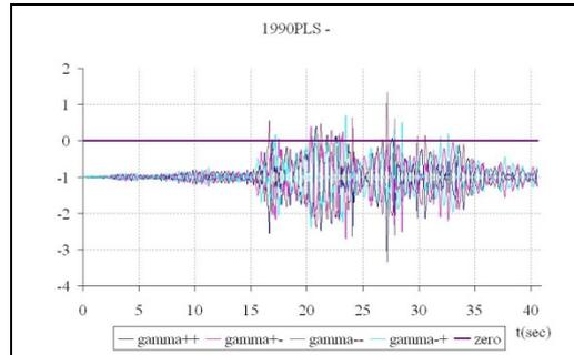
Fig. 5.3. Vertical accelerograms derived for the corners of building of Fig. 2.3, for the event of 1990.05.30
