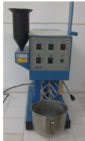
Fig. 1. Mortar mixer with manual/automat functions according to SREN 196-1 produced by ELE company
