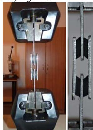
Fig. 8. *The shear test of elastomer* [7]
