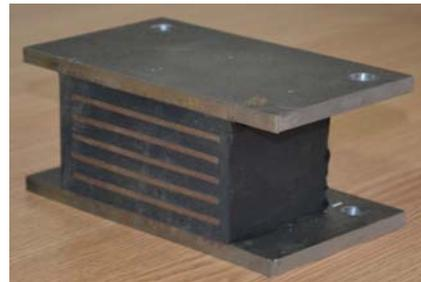
Fig. 10. *The elastomeric bearing*
