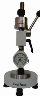
Fig. 2. *The Shore hardness tester* [4]
