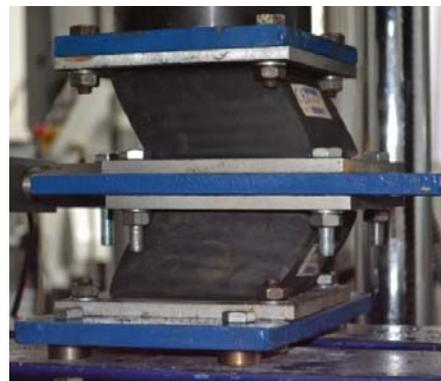
Fig. 11. *The elastomeric bearing displacement*
