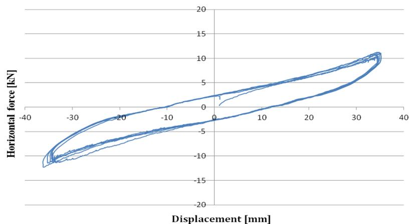
Fig. 12. *The force-displacement curves of elastomeric bearings*
