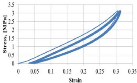
Fig. 7. *The stress-strain curves of SBR*
