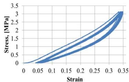
Fig. 6. *The stress-strain curves of BR*
