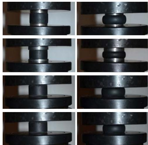
Fig. 3. The compression test of elastomers
