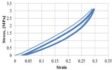
Fig. 5. *The stress-strain curves of NR*
