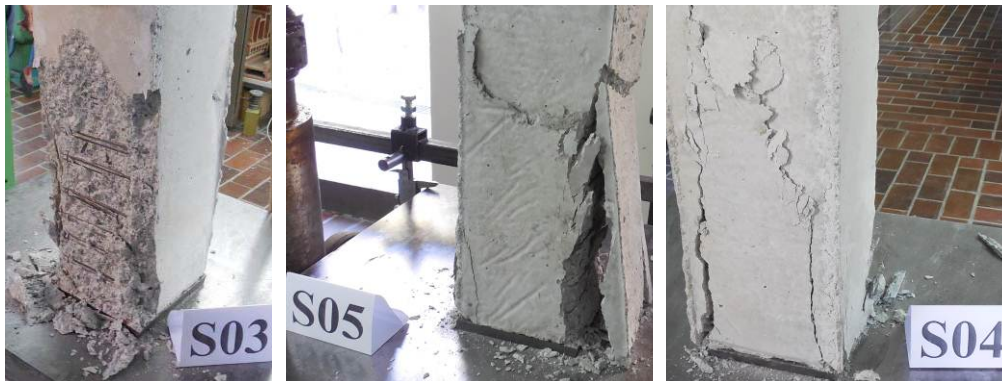
Fig. 5. Column samples of the second group after testing
