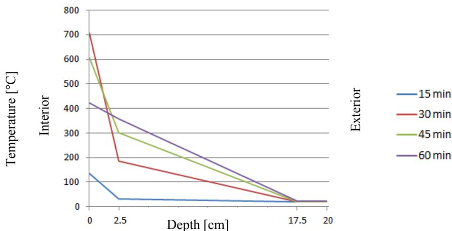
Fig. 6. Temperature profile in the concrete slab
