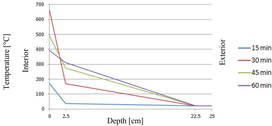
Fig. 6. Temperature profile in the concrete wall
