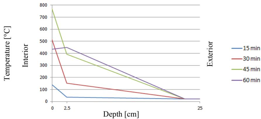
Fig. 7. Temperature profile in the brick wall
