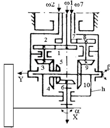
Fig. 10. The kinematic scheme for the angles pair  $\alpha$  -  $\beta$  -  $\gamma$  (2<sup>nd</sup> variant)
