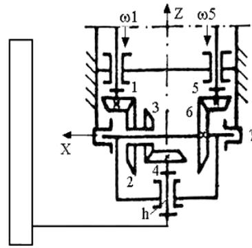
Fig. 6. The kinematic scheme with planetary bevel gears for the angles  $\alpha - \gamma$  (2<sup>nd</sup> variant)
