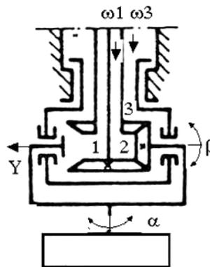
Fig. 4. Kinematic scheme with symmetrical differential for the angles  $\alpha$  -  $\beta$  (variant 2)
