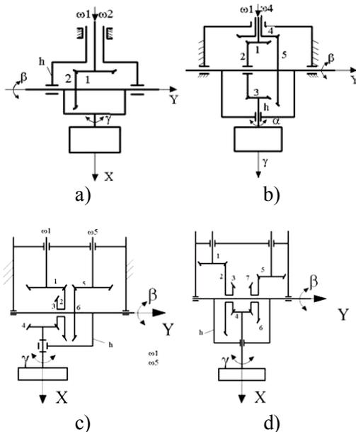
Fig. 8. The kinematic scheme with bevel gear mechanism for the angles  $\beta - \gamma$
