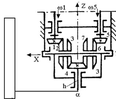
Fig. 7. The kinematic scheme with planetary bevel gears for the angles  $\alpha - \gamma$  (3<sup>rd</sup> variant)
