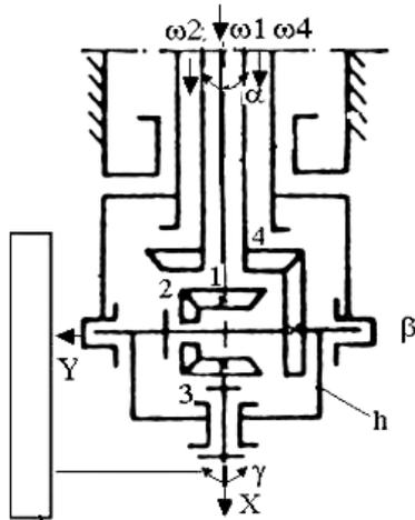
Fig. 9. The kinematic scheme for the angles pair  $\alpha$  -  $\beta$  -  $\gamma$  (1<sup>st</sup> variant)
