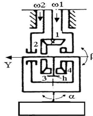
Fig. 3. Kinematic scheme with symmetrical differential for the angles  $\alpha$  -  $\beta$  (variant 1)
