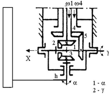
Fig. 5. The kinematic scheme with planetary bevel gears for the angles  $\alpha - \gamma$  (1<sup>st</sup> variant)
