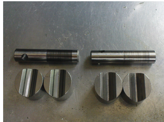
Fig. 8. Scuffed pins and vee-blocks
