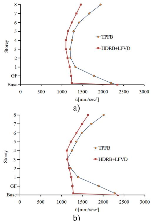
Fig. 5. The mean absolute accelerations of the isolated structure, with HDRB+LFVD system and with TPFB system:
