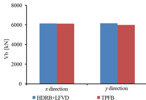
Fig. 7. The mean base shear forces
