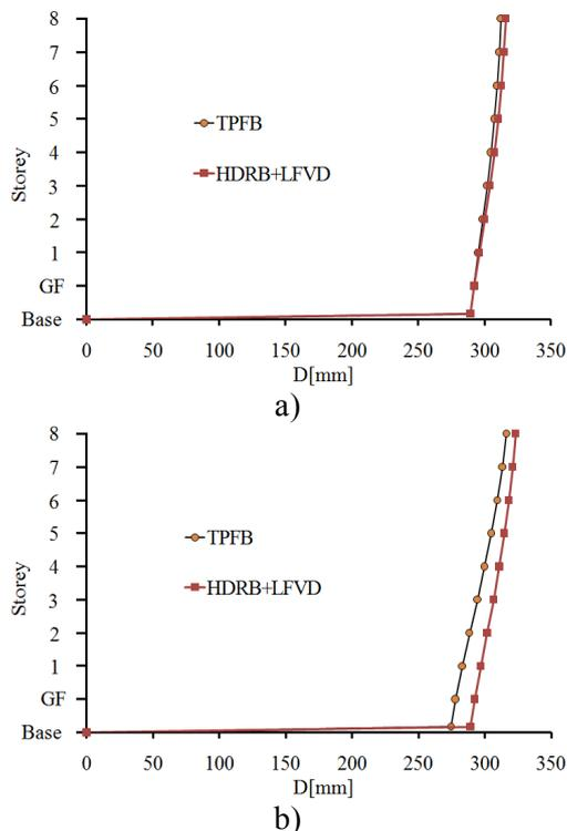
Fig. 4. The mean relative displacements of the isolated structure, with HDRB+LFVD system and with TPFB system:
