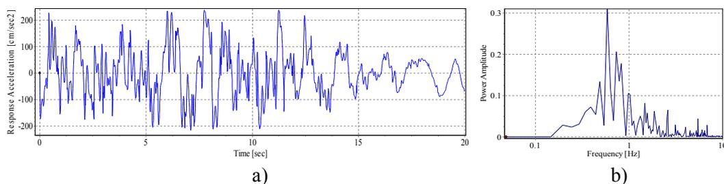
Fig. 3. Artificial accelerogram (a) and power spectral density of the accelerogram (b)
