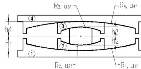
Fig. 2. Schematic configuration of a triple pendulum friction bearing
