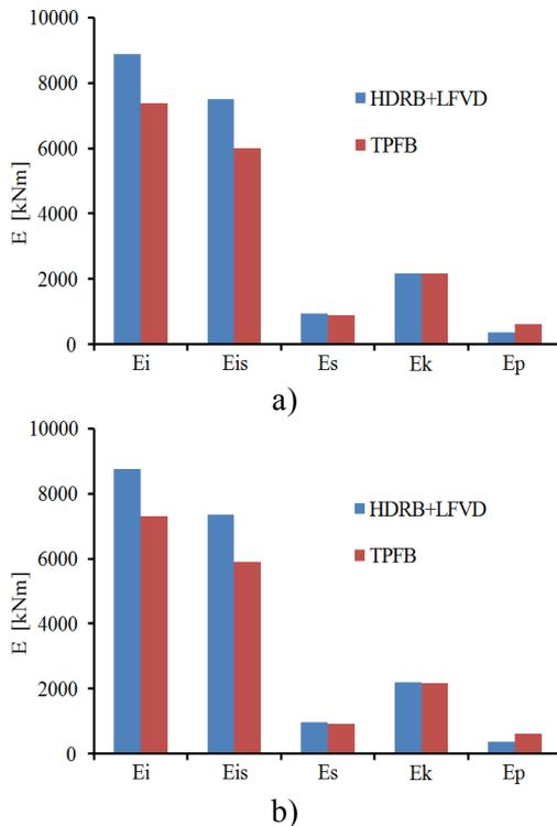
Fig. 6. The mean energies of the two isolation systems: a) x direction; b) y direction
