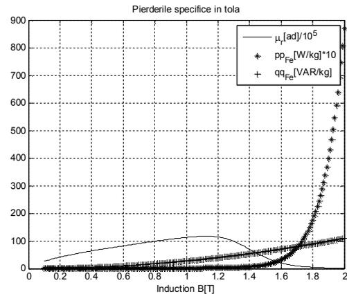
Fig. 8. Characteristics of iron steel
