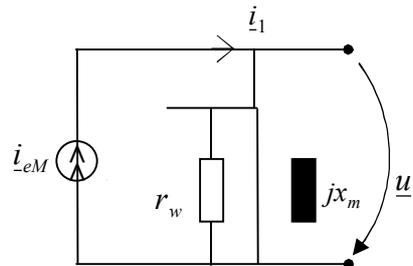
Fig. 5. Electric circuit equivalent scheme of permanent magnet machine
