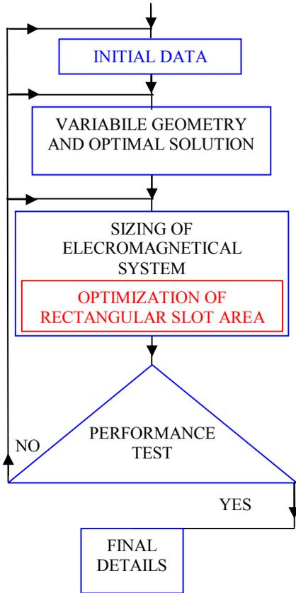
Fig. 3. Improved algorithm for generator design
