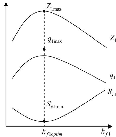
Fig. 2. Graphics of slot area, slot number per pole and phase and total slots
