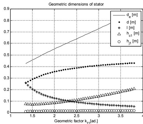
Fig. 9. Geometric dimensions of stator
