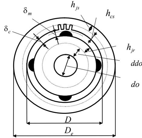
Fig. 4. A cross section on permanent magnet synchronous machine
