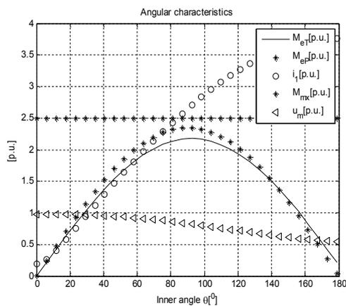
Fig. 7. Estimated angular characteristics
