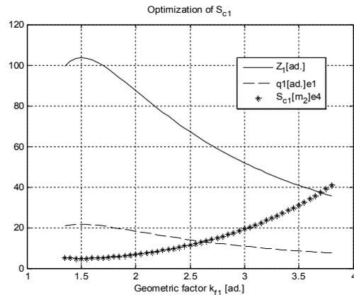
Fig. 13. Optimization of slot area
