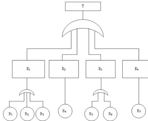
Fig. 4. *Faults tree for the cold monojet water meter**Probabilities of failure for the minimal cuts* Table 1
