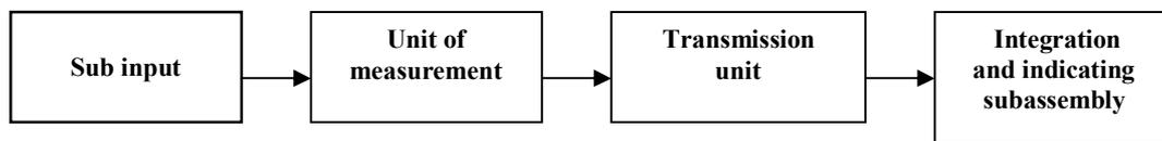
Fig. 1. *Logical scheme of reliability of a cold monojet water meter*
