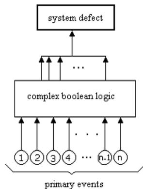
Fig. 3. Scheme of principle of a faults tree
