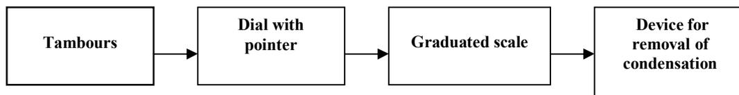
Fig. 2. *Integration and indicating subassembly*
