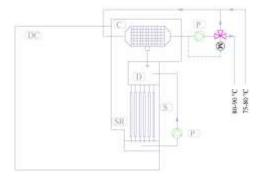
Fig. 3. First proposal for heat recovery from servers, with pump circulation
