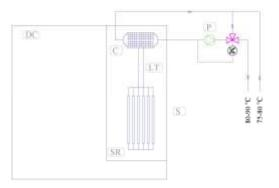
Fig. 4. Second proposal for heat recovery from servers, with thermosiphon, which includes: Data Center - DC, Server Plates - S, Pump Liquid – P, Liquid Distributor – D, Condenser – C, Liquid Tube with Distributor – LT, Closed Server Room – SR.
