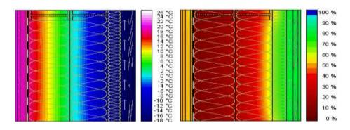
Fig. 3. Detail of the structure wall, temperature and humidity profile for case 2[7]
