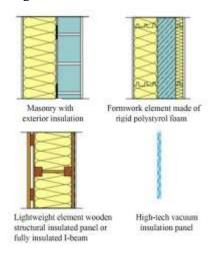
Fig. 1. Wall constructions suitable for passive house standard [6]
