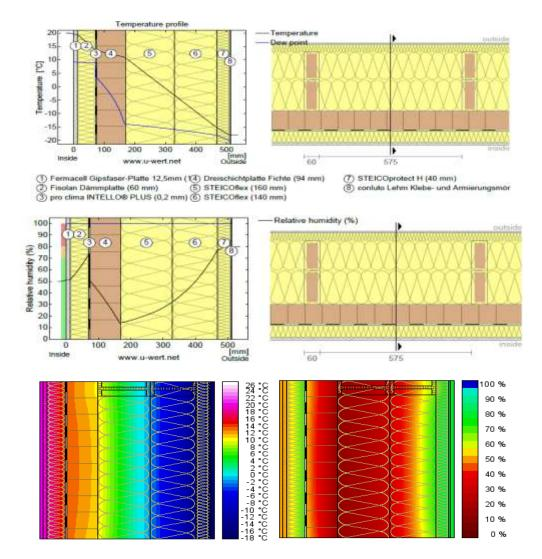
Fig. 4. Detail of the structure wall, temperature and humidity profile for case 3 [7]
